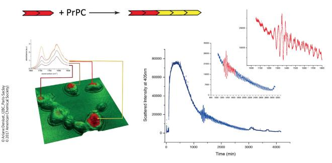
Fibers of prion protein (PrPC) characterised by AFM coupled to infrared spectroscopy (left panel). The fibers' disassembly kinetics (right panel).
